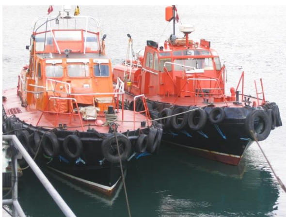
Treffry and Gore Point (the prototype for the Thames class) alongside each other. Treffry had a flying bridge and upper steering position
