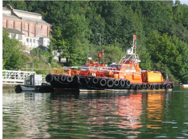
Treffry and Gore Point (the prototype for the Thames class) alongside each other. Treffry had a flying bridge and upper steering position
