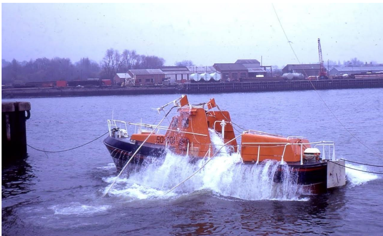
“Rotary Service” righting test which all lifeboats go through
