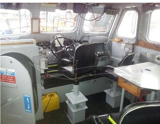
The wheelhouse and the lower steering position with water tight door accessing for'd cabin
