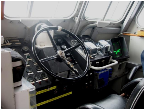
The wheelhouse and the lower steering position with water tight door accessing for'd cabin
